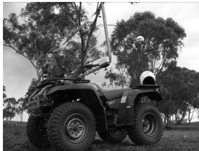
(c) ATV-mounted AOS (with GPS and datalogger) for on-the-go surveying.
